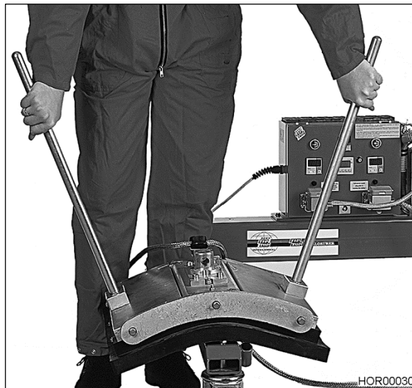
Bild 12 Replacing the heating plate contour segments
