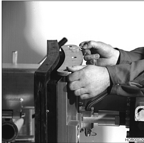
Bild 11 Replacing the heating plate contour segments
