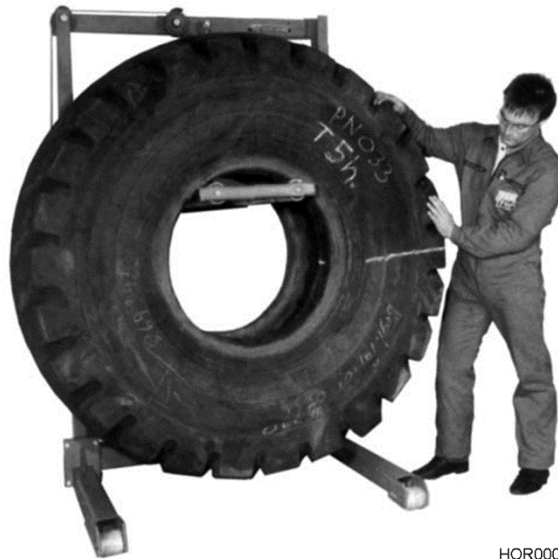
Bild 12 Hooking the tyre into the repair stand
