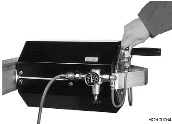
Bild 22 Operating the control unit/closing the pneumatic pressure unit
