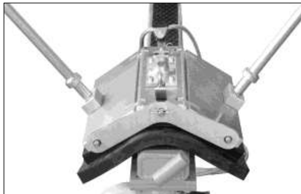
Bild 14 Replacing the heating plate contour segments
