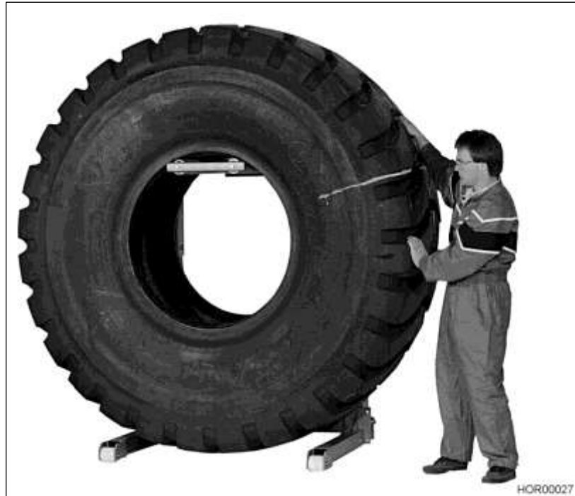
Bild 12 Hooking the tyre into the repair stand
